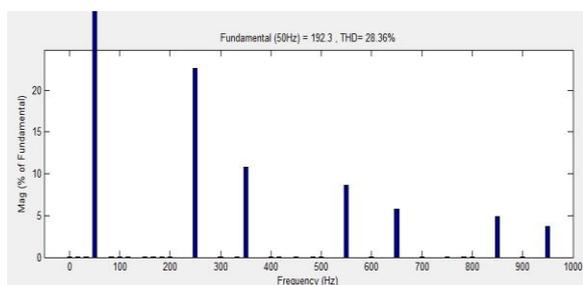
Figure 10: THD value in line current without DSTATCOM.
