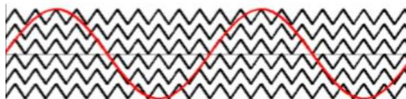
Figure 7: Level Shifted (IPD) seven level for CMC.
