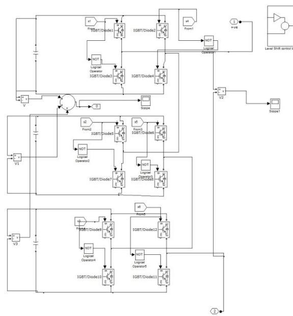
Figure 2: Seven level Cascaded H-Bridge Inverter per phase in DSTATCOM.
