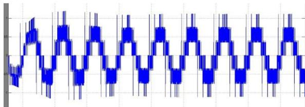
Figure 17: Seven level-Phase shift inverter result.
